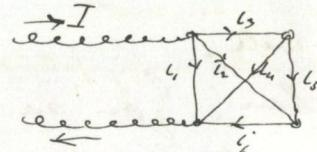
Current  $I$  from battery meets vertex of a square formed by 4 wires. There are diagonal wires. Find current in each part. I find  $l_3 = l_6 = \frac{I}{4}$ , the other is involve  $\sqrt{2}$ .
